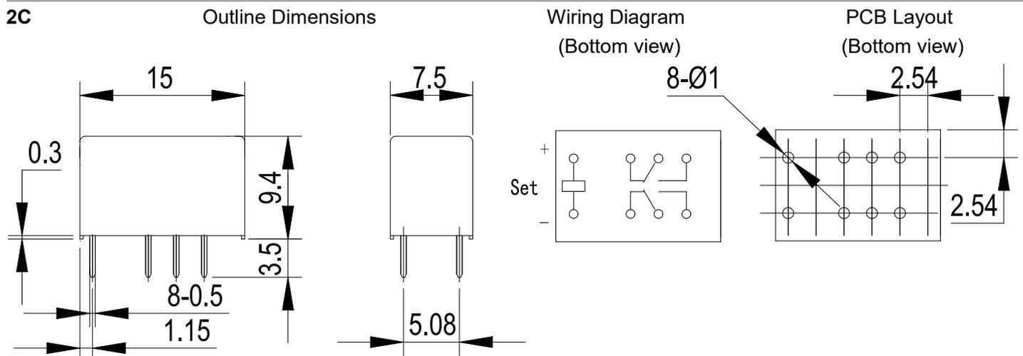
Remark:(1)In case of no tolerance shown in outline dimension:outline dimension≤1mm,tolerance should be±0.2mm;outline dimension >1mm and <5mm,tolerance should be ±0.3mm;outline dimension≥5mm,tolerance should be ±0.5mm.
