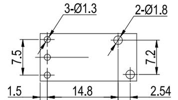
Remark:(1)In case of no tolerance shown in outline dimension:outline dimension $\leq$ 1mm,tolerance should be $\pm$ 0.2mm;outline dimension  $>$ 1mm and  $<$ 5mm,tolerance should be  $\pm$ 0.3mm;outline dimension $\geq$ 5mm,tolerance should be  $\pm$ 0.5mm.
