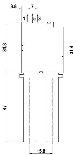
Remark:(1)In case of no tolerance shown in outline dimension:outline dimension $\leq$ 1mm,tolerance should be $\pm$ 0.2mm;outline dimension  $>$ 1mm and  $<$ 5mm,tolerance should be  $\pm$ 0.3mm;outline dimension $\geq$ 5mm,tolerance should be  $\pm$ 0.5mm.
