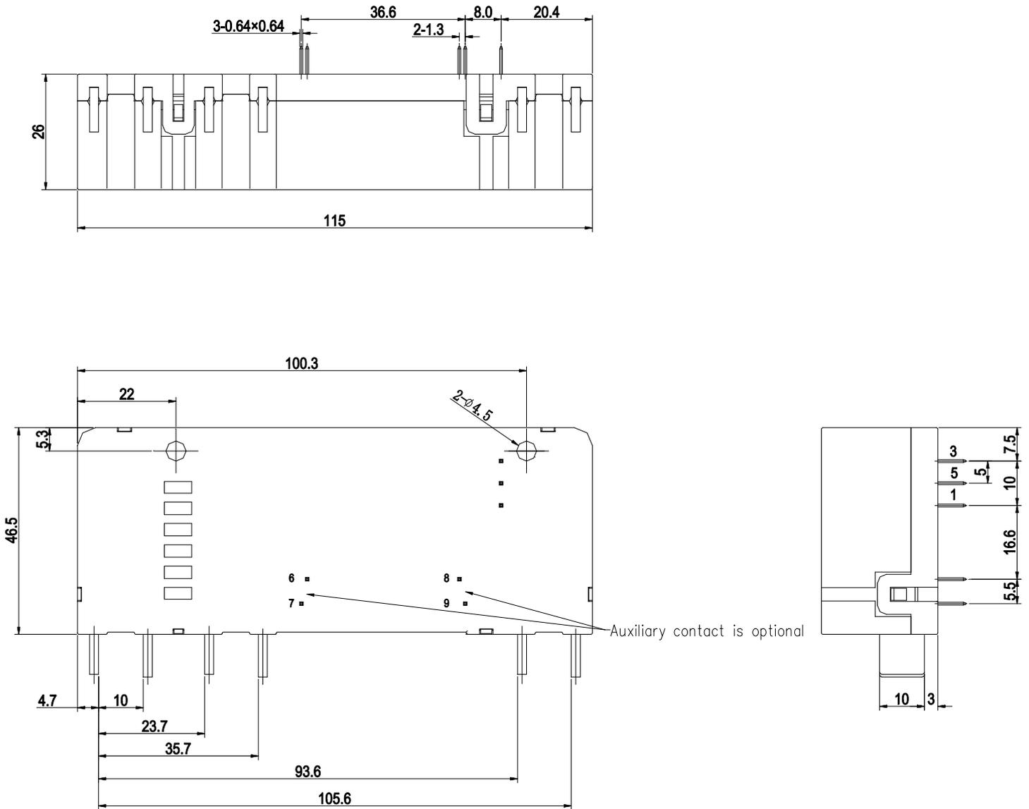
Remark: (1) In case of no tolerance shown in outline dimension:outline dimension≤1mm,tolerance should be±0.2mm;outline dimension >1mm and <5mm,tolerance should be ±0.3mm;outline dimension≥5mm,tolerance should be ±0.5mm.
